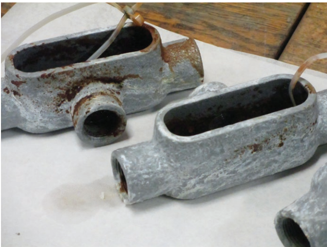
Representative samples of old Duraloy ® paint after 1,000 hours of exposure
