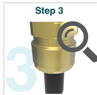
Step 3 The backnut should be level with the marking guide corresponding to its diameter – this can be visually inspected and adjusted as necessary
